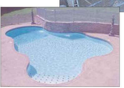
A retaining wall can be added simply by stacking forms and placing the concrete at the same time as the pool wall.
